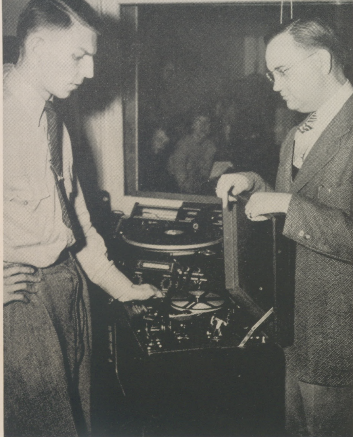
Dick Shoemaker, (top, left) student assistant, and Norman Dohn examine the newest piece of equipment acquired for the radio laboratory. It's a portable tape recorder. The recorder is an excellent training device for radio students as well as for students taking courses in speech and foreign languages. Each spool of tape, which resembles a movie film, will record thirty minutes of music or conversation.
