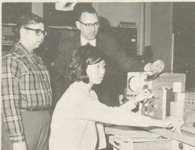
Phillip Barnhart (center) shows students Dennis Lohr of Alum Bank, Pennsylvania and Anna Chen of Hong Kong, the use of the new gamma-ray spectrometer to observe the radiations from a radioactive source.
