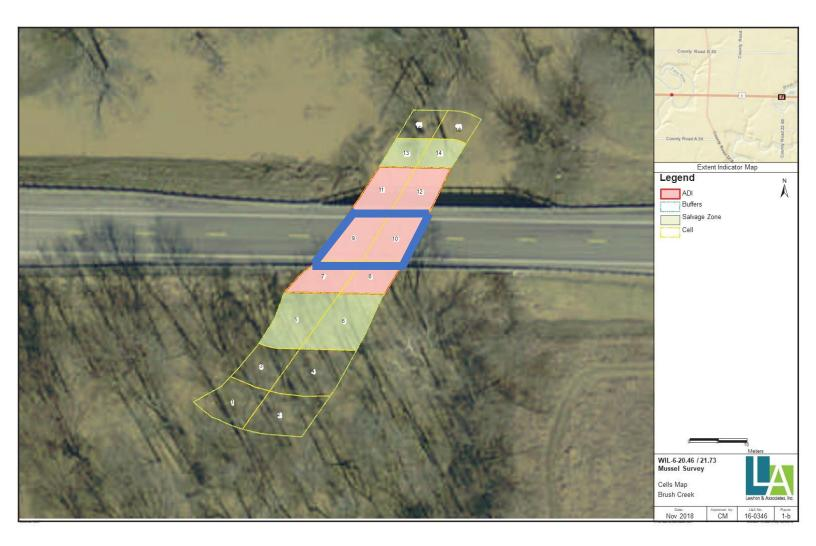
Figure 3. A typical survey layout divided by cells. Cells are labeled and arranged from Downstream (1-6), Area of Direct Impact (7-12); with includes cells under the bridge, and Upstream (13-16). The thicker line is the area that was depicted as the area underneath the bridge (9-10).
