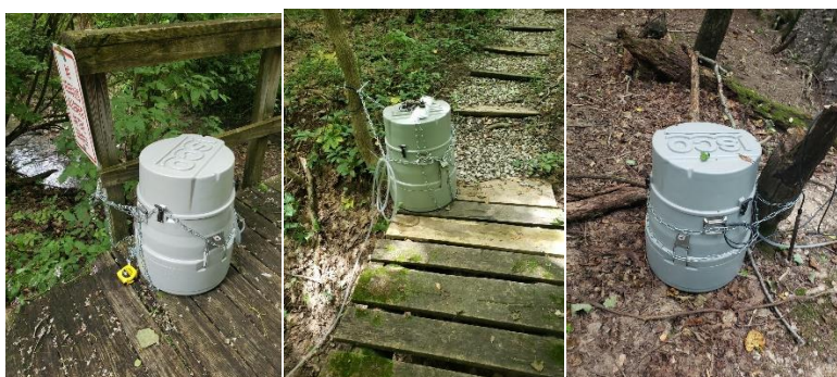
Figure 1: From left to right- Installation of the ISCO water sampler at suburban location, organic location, and commercial exposure location.
