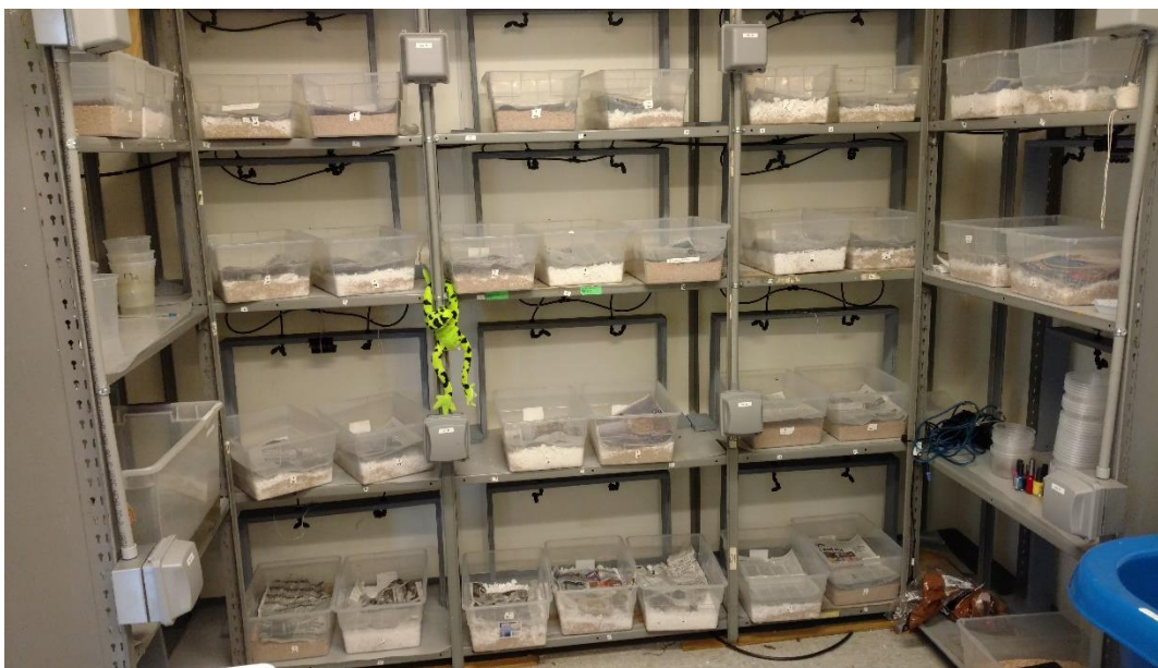
Figure 1. Setup of bins in laboratory space. Replicates for each treatment were stored in plastic bins, each with the same volume of 60900 \text{ cm}^3 . Each replicate was placed randomly on the shelves.
