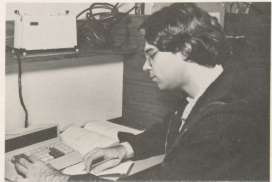
Mike Ziegler, a mathematics and physics major, is shown at the controls of the Wang calculator. The Center provides three control consoles for the calculator, which uses squares, square roots, logs, powers, and a small memory bank, so that the operator can recall the numbers he has submitted.
