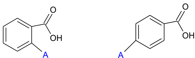
Figure 1. Ortho-substituted benzoic acid (left) is more sterically hindered than para-substituted benzoic acid (right).
