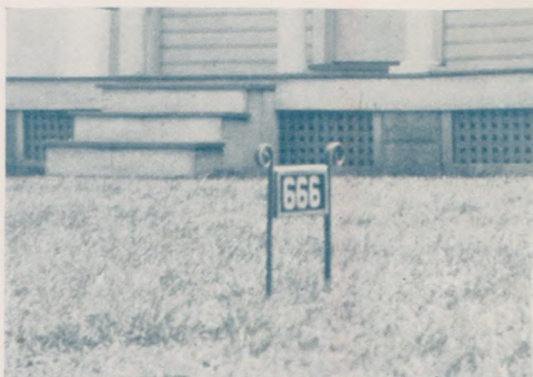
FIGURE 2—Typical double-faced house number. Letters 2½ inches. Taken at 150° angle from distance of 30 feet.
