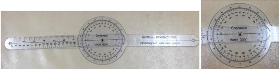
Figure 1. Standard plastic, hand-held goniometer with 1 degree markings
