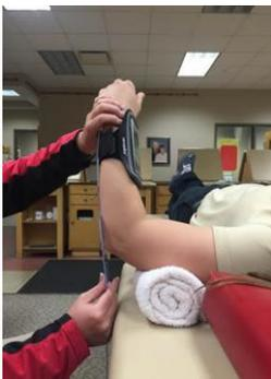
Figure 7. Simultaneous measurement with inclinometer app and goniometer
