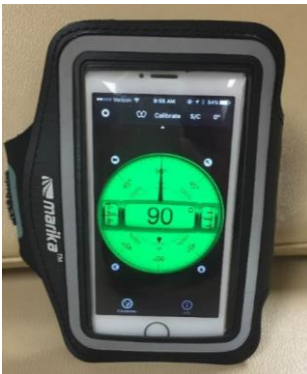
Figure 2. Smartphone application "Clinometer" and activity band
