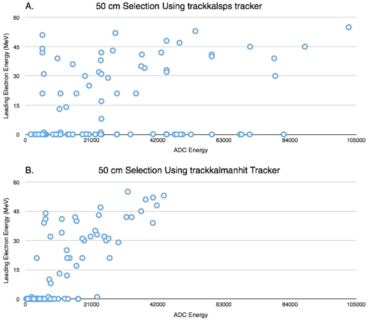
**Fig. 16:** The reconstructed vs. truth energy plots using the trackkalsps tracker, top, and the trackkalmanhit tracker, bottom. As can be seen the trackkalsps tracker seemed to leave behind a large number of excess hits, artificially increasing some of the candidate energies. However, both processes still suffer from a large number of low-Energy false-positives, and several, low energy candidates.
